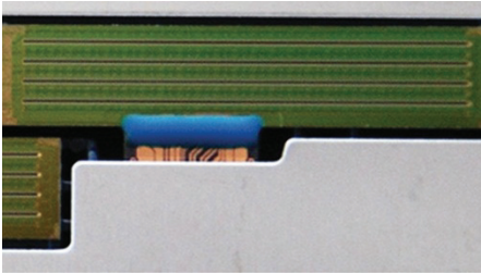
Figure 5: Detail of an HP Thermal Inkjet die
