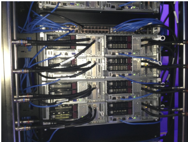
Front IO of Supermicro®'s FatTwin™ SYS-627R2-FT+ with Cool IT Liquid Cooling Cool IT Rack DCLC™ AHx System
